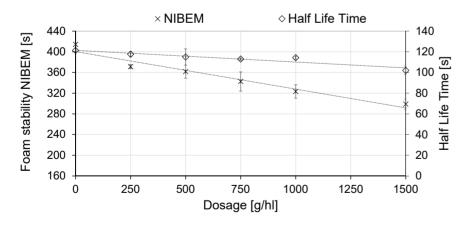
Fig. 5 Foam stability acc. to NIBEM and Steinfurth (0–1500 g/hl for type 90 pellets)
